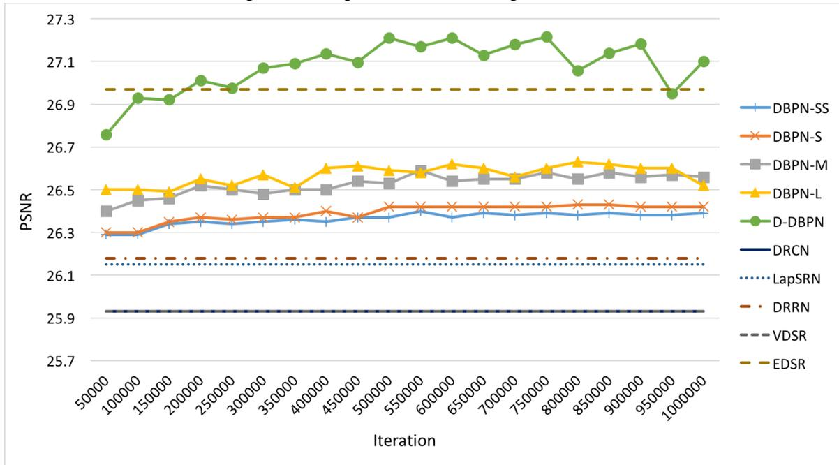
Figure 3. Convergence curve for 8x enlargement on Set5.
