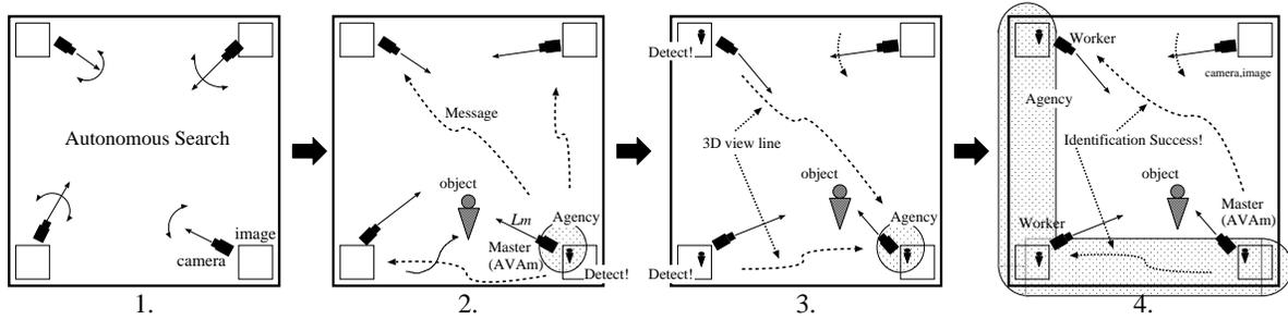
Figure 1. Object tracking system by multiple AVAs
