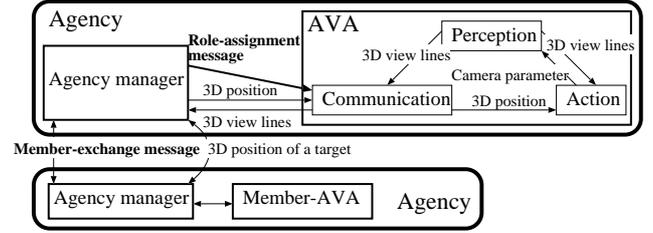
**Figure 4. Elements of communications at and between the three layers.**
