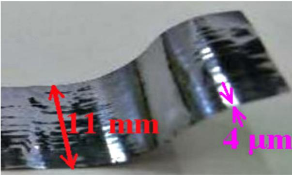
(a) 4  $\mu$ m-thick steel sheet
