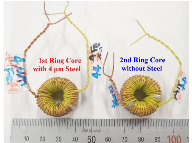
Fig. 3. Two ring cores with same dimension and number of turns of copper coils; left: first ring core with considered steel part; right: second ring core without steel part
