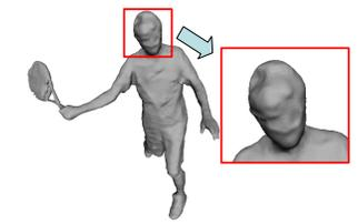
Figure 16. 3D mesh obtained only from 12 zoom-out images.
