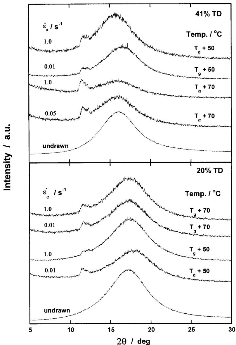
Fig. 3. WAXD patterns of two different TD content copolymers before and after elongation at various Hencky strain rates of two different temperatures.
