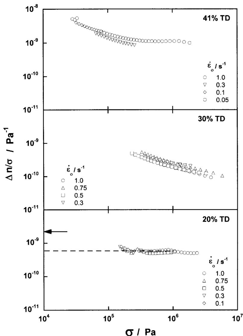
Fig. 2. Stress optical coefficient  $C(\dot{\epsilon}_0; t) \equiv \Delta n(\dot{\epsilon}_0; t)/\sigma(\dot{\epsilon}_0; t)$  for indicated copolymer at  $T_g + 50^\circ\text{C}$ . The dashed line indicates the constant  $C(t)$  of 20% TD and the arrow indicates the reported value of  $C(t)$  for LDPE.
