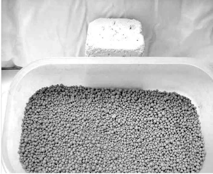
Figure 10. Picture of the ceramized product Pellexpended®. At the top of the picture, there is a piece of light concrete produced with this material.
