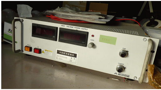
Fig. 1: High Voltage Power Supply
