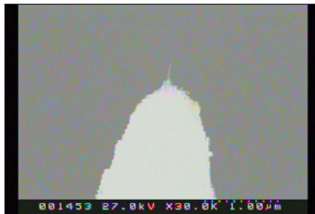
Fig. 1 SEM micrograph of an STM probe tip attached with a bundle of SWNTs.
