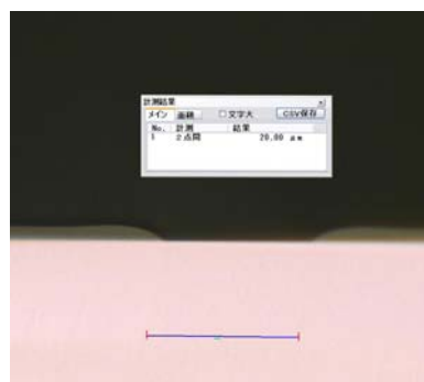
Fig.5 Optical microscopic image of photoresist (TSMR-V90) from side view
