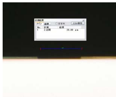
Fig.6 Optical microscopic image of photoresist (AZ1500 3.8cp) from side view
